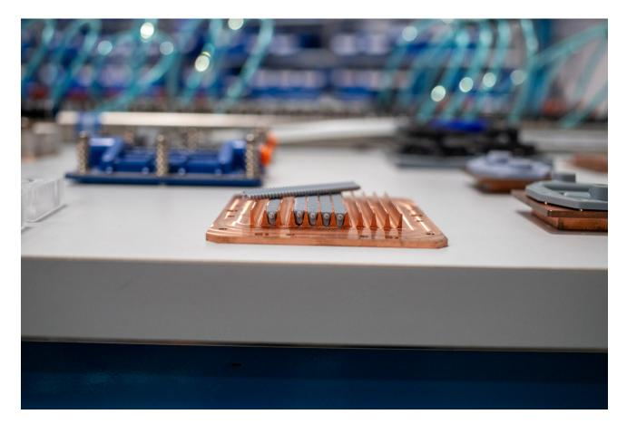
The coolant, water in this case, flows through the cold plate's internal channels, carrying the heat away from the component. This process ensures efficient cooling, maintaining optimal operating temperatures and improving the performance and reliability of electronic devices.
