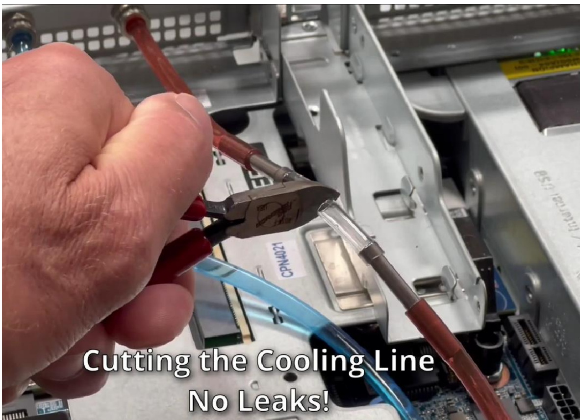
Figure 10: Screenshot from a video showing a cooling line being cut on a Dell R760xp. As soon as the coolant loop is exposed to air, the liquid vacates from both sides, eliminating the risk of coolant leaks through negative pressure technology. Watch the full video here:
