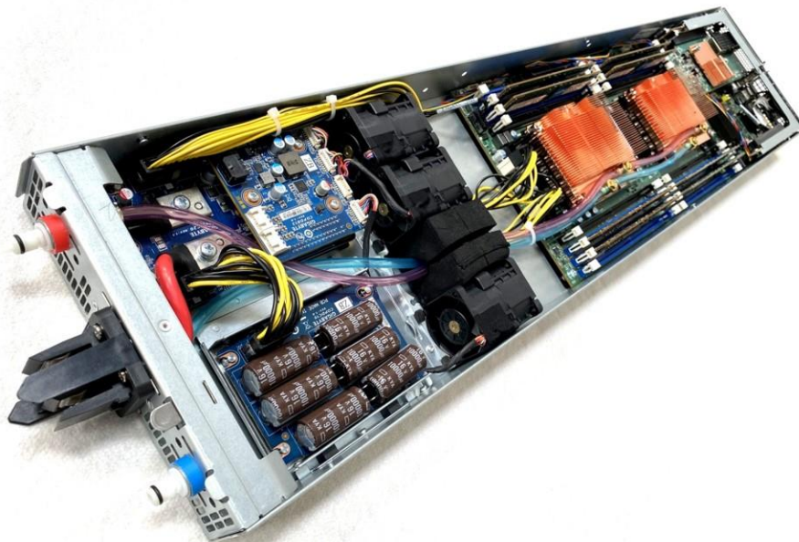
Figure 2: An OCP node featuring copper cold plates specifically for direct-to-chip liquid cooling.
