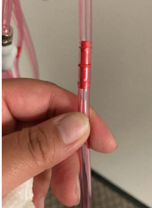
Figure 15: Sonic Venturi flow limiter on return side
