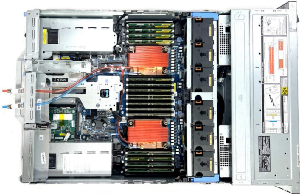
Figure 3: A Dell R760xp server modified for direct-to-chip liquid cooling, with copper cold plates prominently visible.
